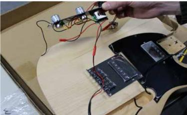
Connect the cables of the pickups to the cables which are on the switch. The final black wire, the ground, will need to be fed through the hole and sit under the bridge. It does not need to be soldered, as long as it is touching the bottom of the bridge it will work.
