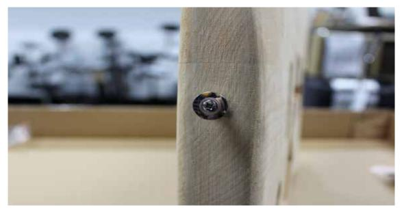
Screw the strap buttons into the pre-drilled holes at the bottom edge of the body and at the tip of the upper horn of the body.
