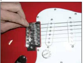
Once the desired action is achieved, all that remains is to set the vibrato tension and intonation. After tuning up all the strings, the spring claw may need tightening (or slackening) in the rear cavity to make the vibrato system "float" (note: some players prefer that the bridge lies completely flat against the body).
