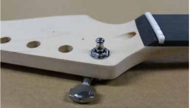
Fix the retaining screw through the loop on the rear of the gear housing into the pilot hole to hold the tuner inposition. Then tighten the nut on the front face of the tuner until it is firm by using a spanner of the correct size. Repeat this for the remaining five tuners and then fit the two string trees with the one with the taller spacers nearer to the top nut.
