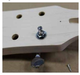
Tighten the nut on the front face of the tuner until it is firm by using a spanner of the correct size. Repeat this for the remaining five tuners.
